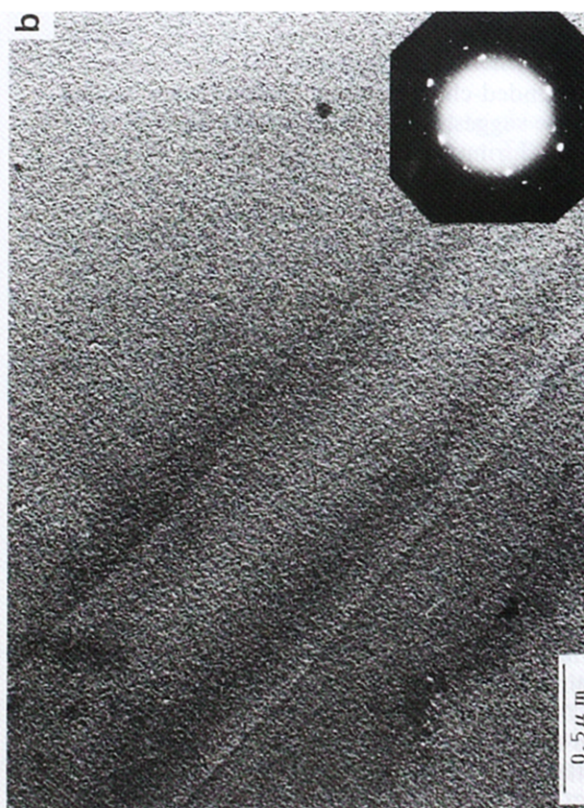
Figure 5 Electron micrographs and corresponding electron diffraction patterns of TPI-1 ( M_w = 3490 ) heat-treated at 350 °C. The dotted circle in (a) shows a 'remnant' of the original droplet-like structure
